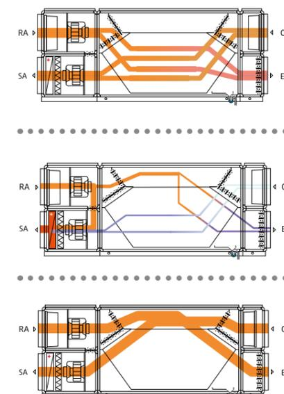
of untreated recirculation air, heated at the condenser and routed into the hall as supply air. If necessary, further heating is carried out with the help of heating coils. During swimming pool mode, the minimum required amount of outdoor air is added as needed.
