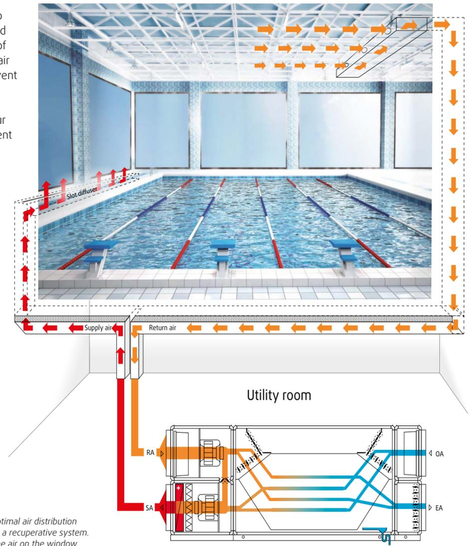
Example of an optimal air distribution system based on a recuperative system. Introduction of the air on the window facades, extraction at the top. The amount of supply and return air is constant.
