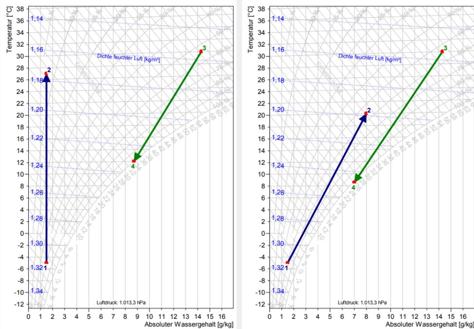
Energetic examination of recuperative and regenerative heat recovery (left) and heat recovery with heat wheel (right). The diagram shows that there is a big difference in the absolute water content between the return air and outside air in the case of low OA temperatures.
