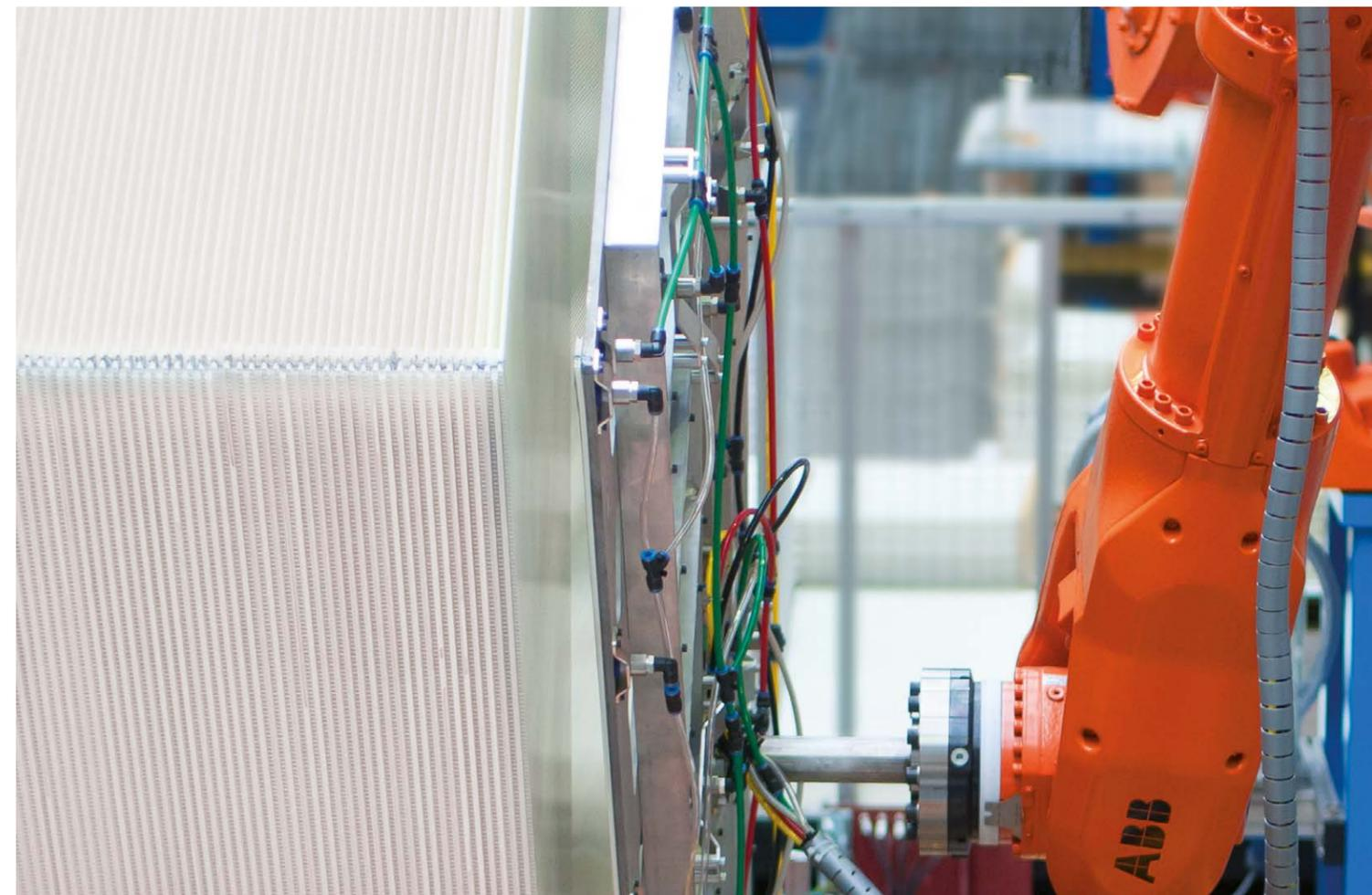
Heat exchanger made of polypropylene, fully automated production.
